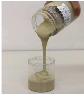
Figure 3. Heavy bentonite-based slurry.
